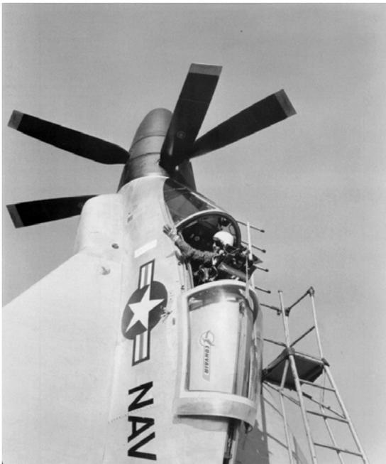
The single pilot sat underneath a cockpit canopy which slid toward the rear. The ejector seat was mounted on gimbals and tilted 45 degrees when the airplane was in the vertical position. Entry to or exit from the cockpit required a special ladder, and was by all accounts rather awkward.
