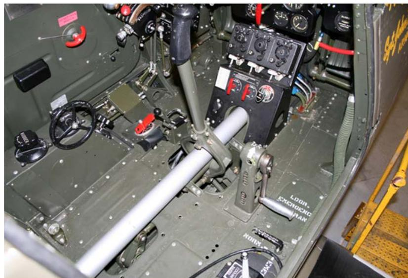
When the airplane first appeared there were many naysayers forecasting doom for a configuration having a 10' drive shaft extension between the engine and its reduction gearbox ....
