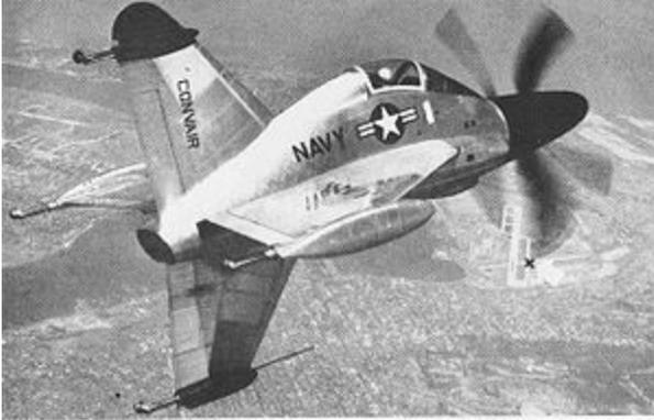
Unfortunately, the XFY-1 was difficult to land because of a poor view of the landing area from the cockpit and the unusual pilot posture. The landing operation would probably have been difficult if not impossible for a pilot of ordinary ability to perform on a small deck aboard ship, especially in rough seas where the deck was pitching and rolling about.
