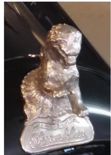
Franklin Rampant Lion radiator mascot. "Radiator" functions as a hood support as all Franklins had air-cooled engines
