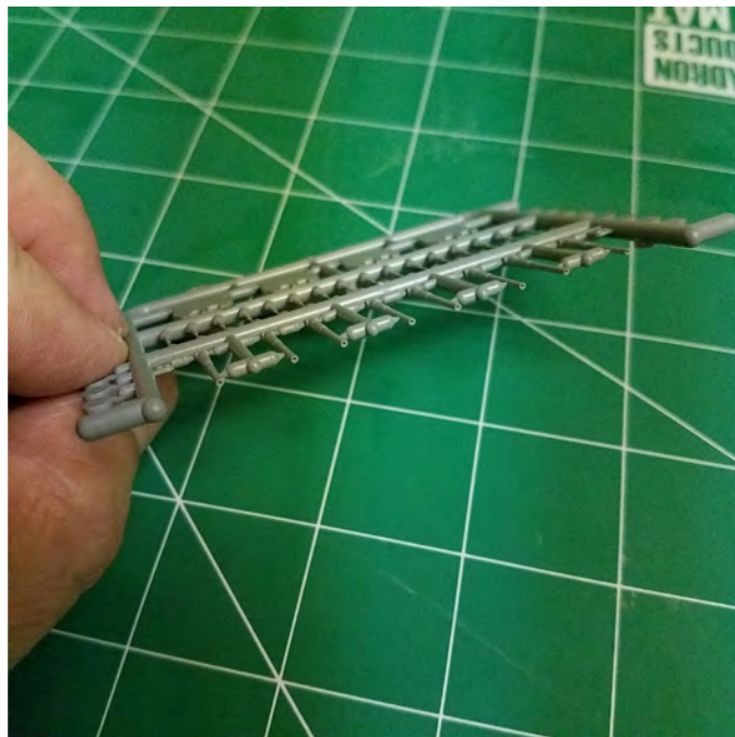
Slide-molding has been used extensively to give hollow items like the stacks and the end of the gun barrels.
