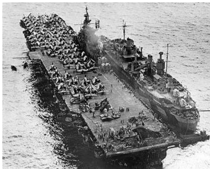
Randolph with Ajax alongside after the kamikaze attack. Note the hole in the deck.
