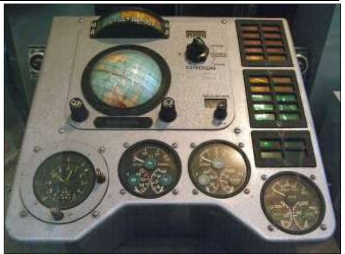
Part of the Vostok 1 instrument panel prominently displaying the "Globus" navigation instrument
