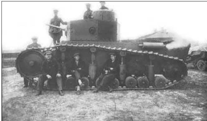
A T-12 is posed on by workers and officers. The eight sided turret is very clear in this image.
