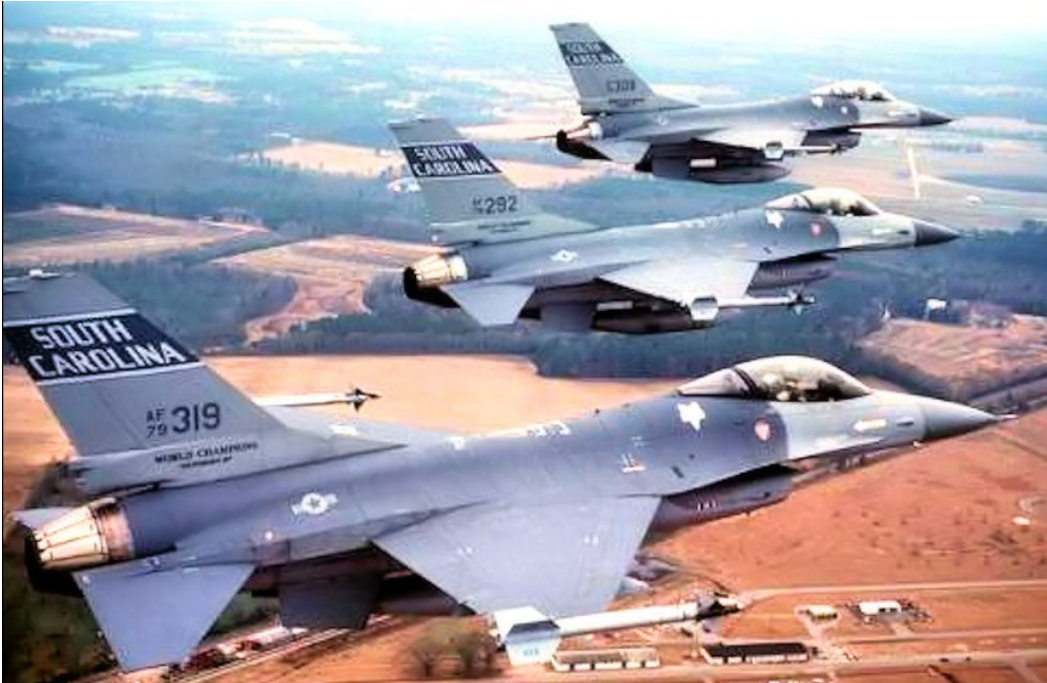
A group of Block 10 F-16's on a mission. Note the Darby Erd-designed tail band and the “World Champions—Gunsmoke ‘89” titles on the tail. Also note the small horizontal stabilizers. (SCANG/USAF)
