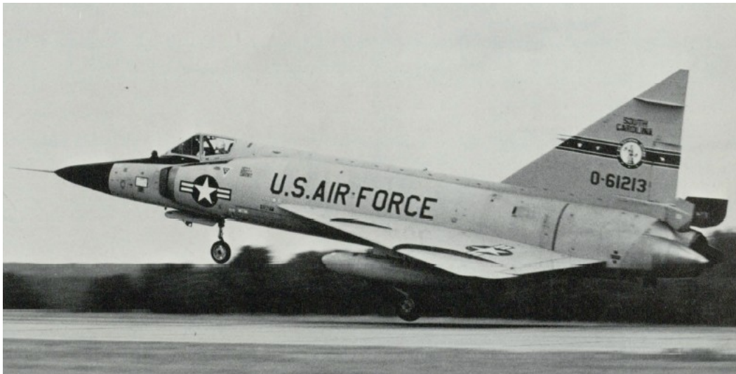
About to rejoin the Earth. Again, note the Case X wing. The radome and anti-glare are black (flat and gloss, respectively). Again, note the IR Sensor. (SCANG/USAF)
