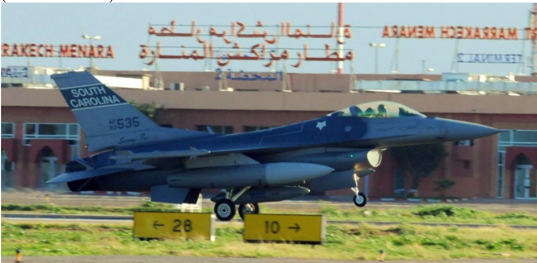
An SCANG Block 52 F-16C touching down in Marrakesh, Morocco. This airplane appears to have the two-color scheme as opposed to the 3-color scheme of the earlier airplanes. Note the white inlet interior. Also note the changes to the typeface on the tail—it is a common font, probably to ease the task of painting. The paint shop probably uses a commercial vinyl cutter to cut the masks, so they simply use the fonts available. (SCANG/USAF)
