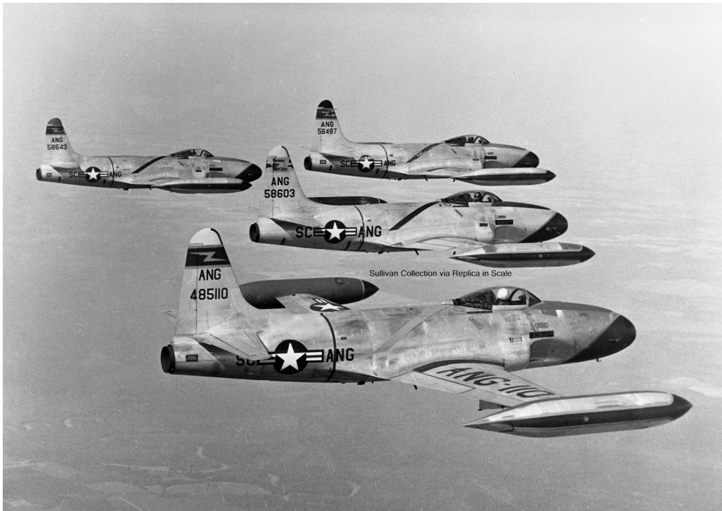
A four-ship of F-80C's. Note the Fletcher wingtip tanks. (USAF Photo/Sullivan Collection via Replica in Scale)
