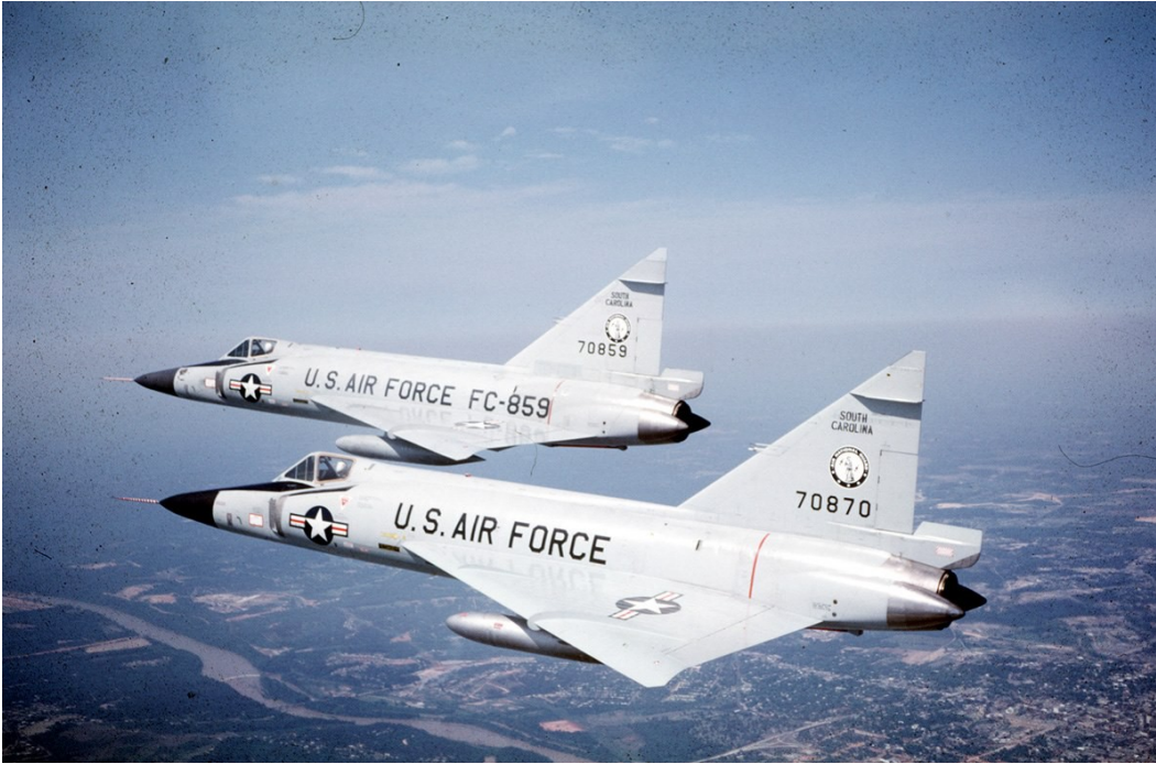
A pair of Deuces. Note the Case XX wings—cambered leading edge, downturned wingtips. Note the lack of Infrared (IR) sensors on the nose in front of the windscreen. (SCANG/USAF)
