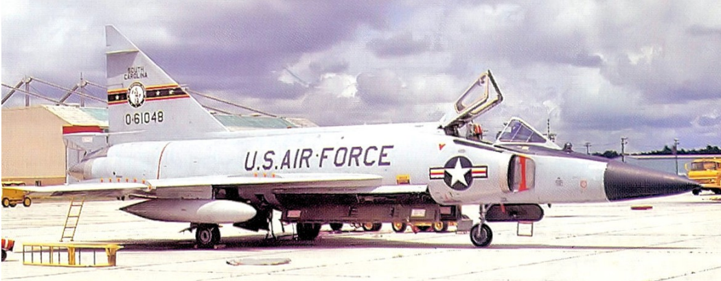
This one has the blue/red band on the tail. Also, note the Case X wing—upturned wingtips and relatively flat leading edge. Here you can also see the IR sensor. (SCANG/USAF)
