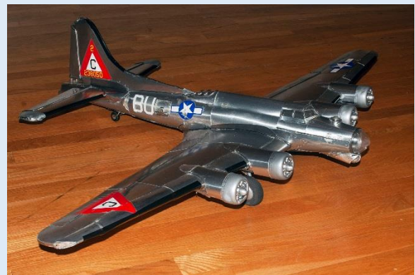
1/32 nd scale B-17 wood model which was covered in thin aluminum sheeting and some other modifications.
