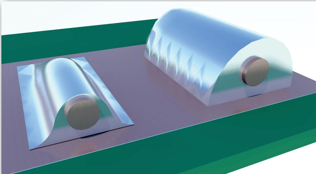
This next illustration shows the range of solder joints one could expect in inspecting a circuit board.
