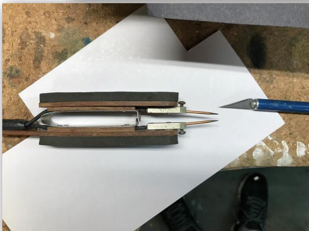
You can't get shocked because the voltage is too low to do much damage, but the tips do get very hot very fast. Not show above is the real magic part: the foot switch. You clamp the parts together with the tweezers, when it looks right, you step on the foot switch to heat the
