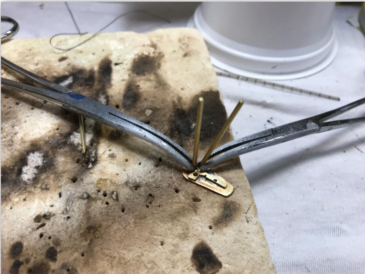
double duty: as work holders AND as a heat sink to catch the heat and divert it before it gets to the old joint. It works!
