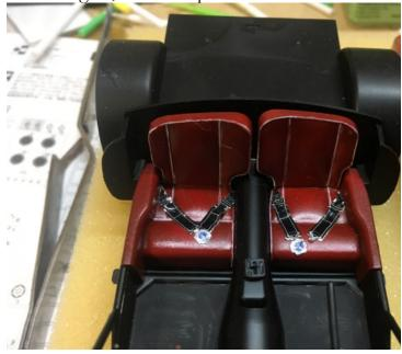
firewall was attached to the chassis, along with the engine mounts, steering linkage, small details, and radiators. I glued the engine in place and moved on to the interior.
