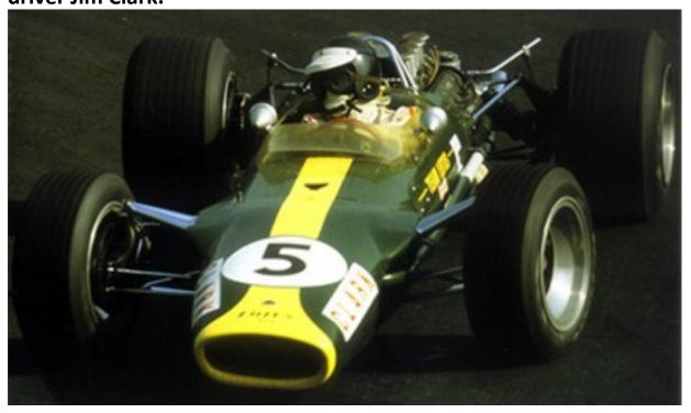
Designed by Colin Chapman, a man whose name in racing history is virtually inseparable from "Lotus", the 49 has been described as an engine, four wheels, and an austere cockpit all fastened together with absolutely the minimum possible structure. Another description was as a high-speed eggshell. Today the wags often call that era of F1 racing as when "....when sex was safe, and driving Formula 1 was dangerous."
