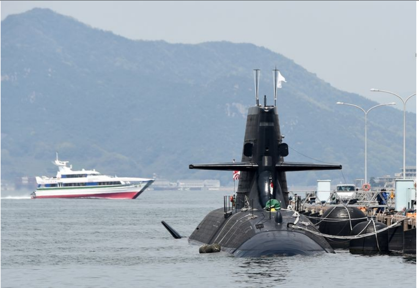
A Sōryū class submarine anchored at the naval base at Kure, Japan. Note x-shaped stern planes emerging from the water at a 45 degree angle.
