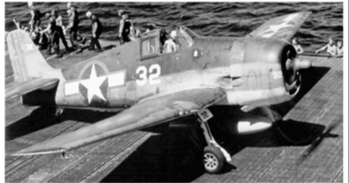
An F6F-3 from VF-16 is about to launch from USS LEXINGTON, CV-16, in November 1943. Known as the "Fighting Airedales," VF-16 was one of the Navy's most successful fighter squadrons during 1943. The Hellcat is painted in the tri-color scheme with Sea Blue on the upper surfaces, Intermediate Blue on the vertical surfaces, and Insignia White on the undersides. What appears to be a red surround on the national insignia is actually a medium blue color that has been hastily applied over the red to cover it after the red surround was ordered deleted from U. S. aircraft. Lt. Alexander Vraciu was VF-16's leading ace with 19 confirmed victories, several of which were scored with VF-6. Vraciu's best day came during the "Marianas Turkey Shoot" when he shot down six Japanese aircraft on June 19, 1944. (National Archives)
