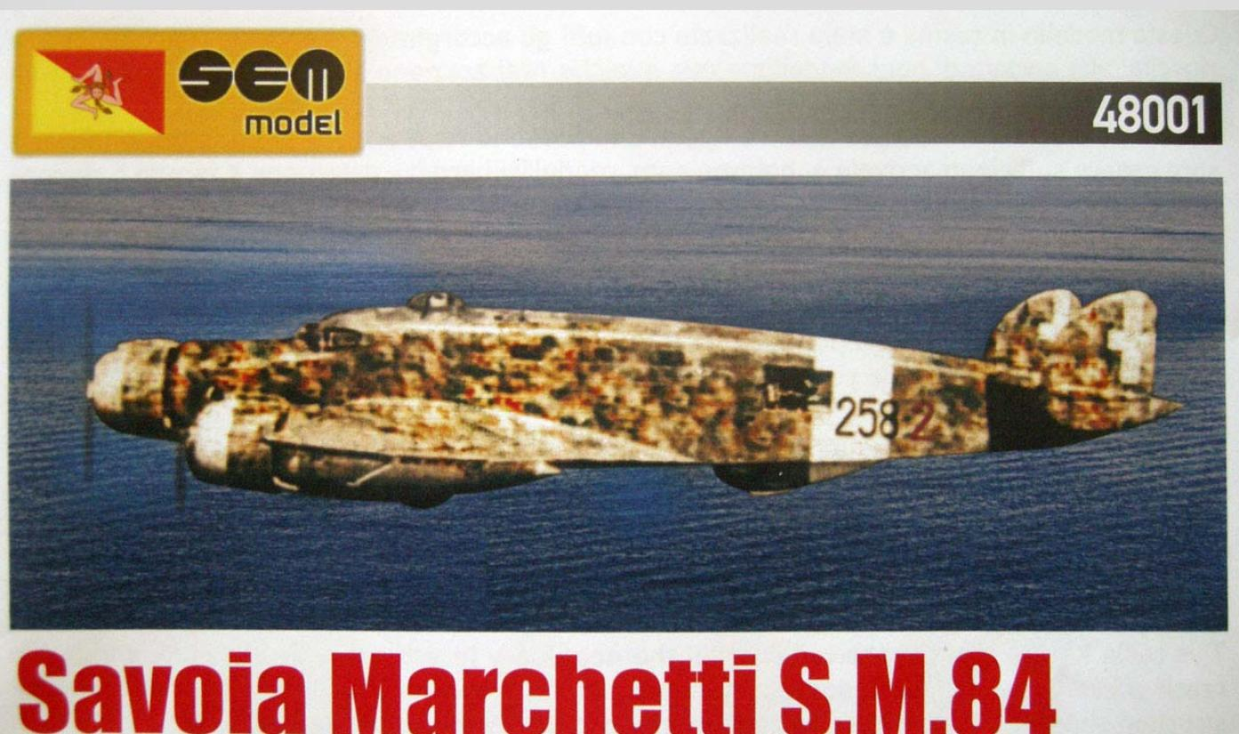
The S.M.84 was designed in 1939 as a replacement for the now aging S.M.79 using a similar wing, but up-rated engines and a re-designed fuselage and more modern internal systems. The first prototype flew on 5 June 1940, just 5 days before Italy's entry into World War II. For more information on the aircraft and it's operational history see [https://en.wikipedia.org/wiki/Savoia-Marchetti SM.84](https://en.wikipedia.org/wiki/Savoia-Marchetti_SM.84).
