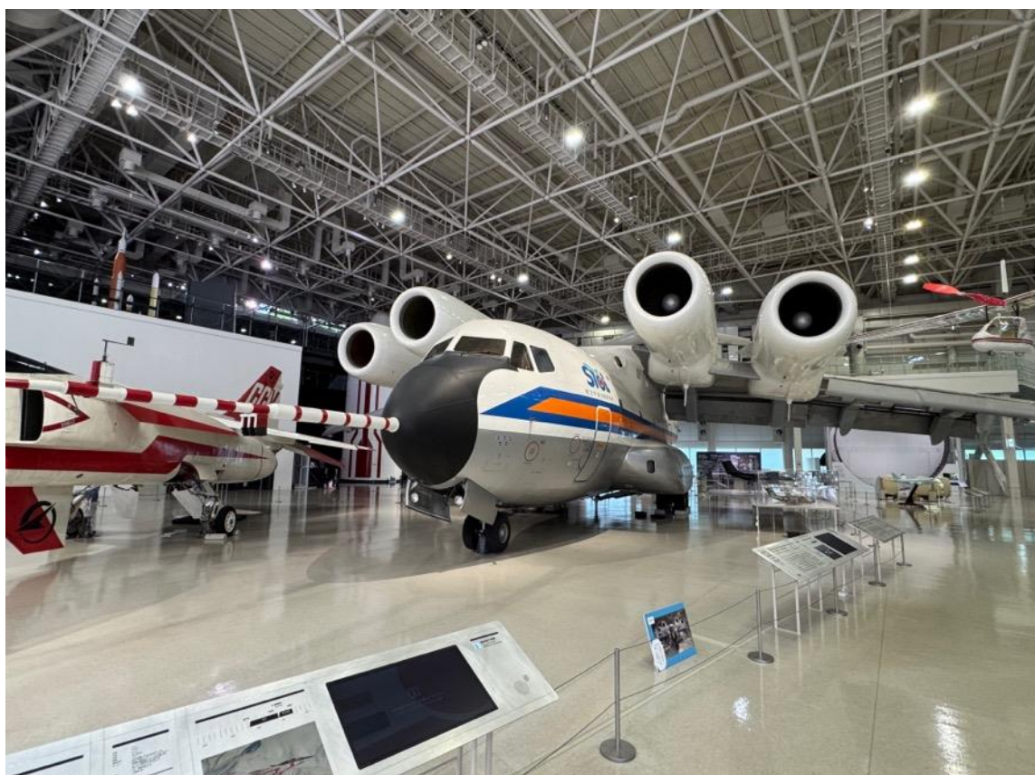
Photo 14: Low-Noise STOL Experimental Aircraft "Asuka"
