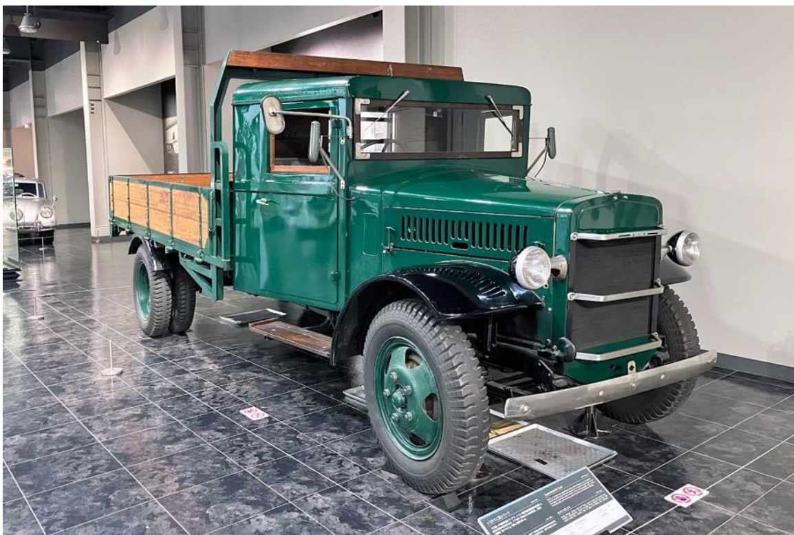
Photo 4: 1945 Toyota Model KC, a simplified wartime spec truck using around 1/3 wood components to save steel
