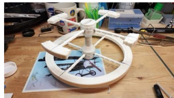
Figure 10: Test fitting the two hub assemblies, which thankfully were keyed to mate only one way. After painting, these would eventually be joined with 2-part epoxy.
