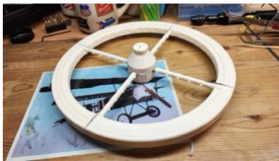
Figure 9: Assembling the completed (solid) ring. Fit was a big problem here – the 4 quarter-arc pieces would not make a perpendicular join at each end simultaneously, nor retain a continuous radius. I worked for the best overall fit possible, and later filled major gaps with epoxy. The slight mispositioning of these segments for best overall fit had adverse implications for the PE wire conduits (or whatever they are) which run radially along each spoke. Don't look too closely...
