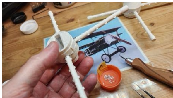
Figure 7: Adding a million triangular reinforcement pieces around the flange at the base of each spoke.
