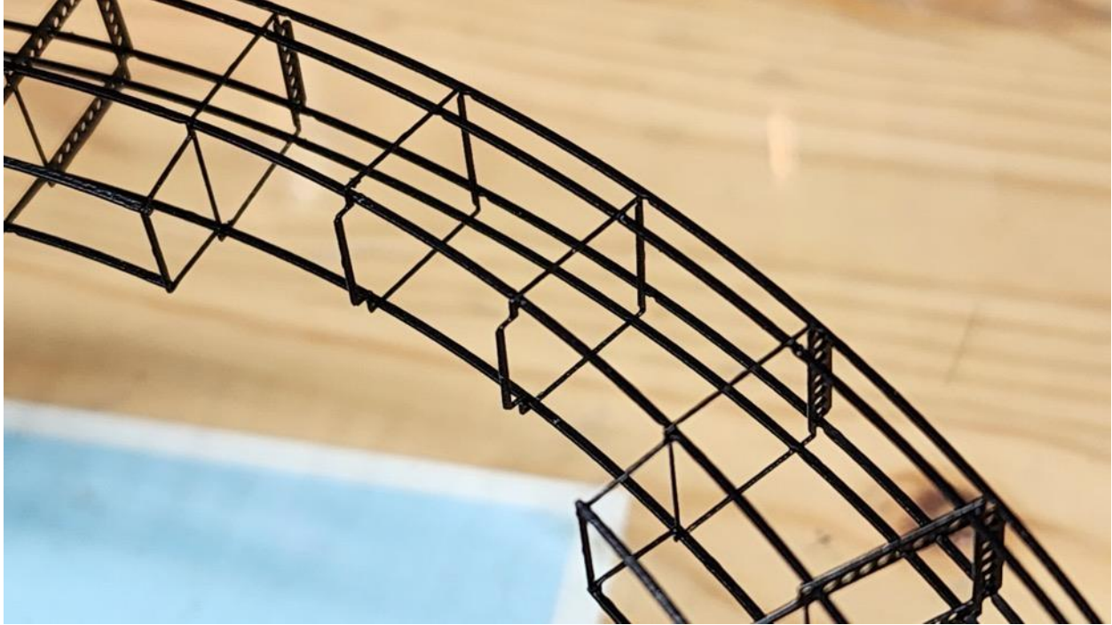
Figure 14: When you look in horror at delicate work you thought was complete, and realize you installed items wrong. Those 2 middle “squares” are upside down – I couldn’t live with the 1 in 1000 viewer who might point this out, so I did surgery.
