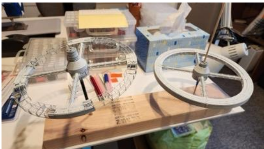
Figure 15: After some touchup and spot repriming with Mission Models MMS-001 Black primer, we move to main painting. I used Mission Models MMP-001 White for the primary coat. The light shade built up over black primer creates shadow effects which highlight the textures of the models (some of which I’d rather not highlight, but I was looking for an overall “busy” surface to emulate the movie with a minimum of effort). It also results in an overall light gray appearance, which I was seeking.
