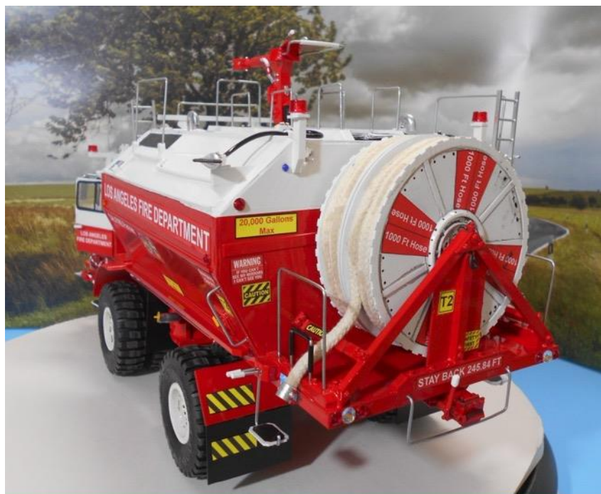
The two 1000 ft reels (2000 ft total) assures the water tank can be filled in many locations if there is a fire hydrant.
