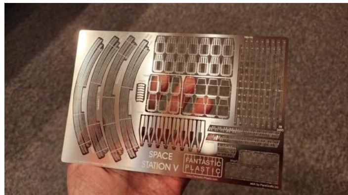
Figure 5: One of multiple sheets of photo-etched (PE) steel, mostly for the exposed truss work of the "under construction" ring. The steel was agreeably strong but cleanup of the multitude (literally hundreds) of stubs was tedious and extremely time-consuming.
