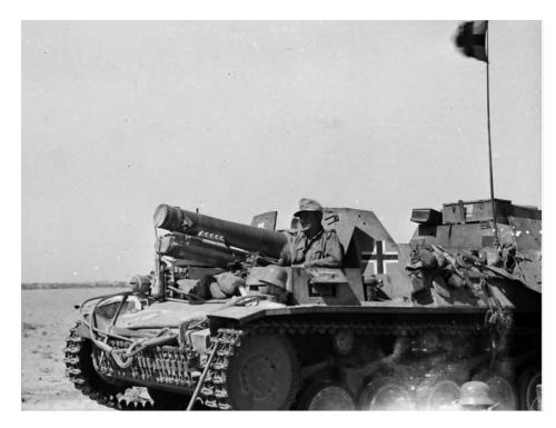
The same gun was mated to the Panzerkampfwagen II chassis in an attempt to drastically lower its height while using a stronger chassis. The prototype used a standard Panzer II Ausf. B chassis when it was built in February 1941, but this was too cramped for use. The chassis was lengthened by 24 inches, which required adding a sixth roadwheel, and widened by 13 inches to better accommodate
