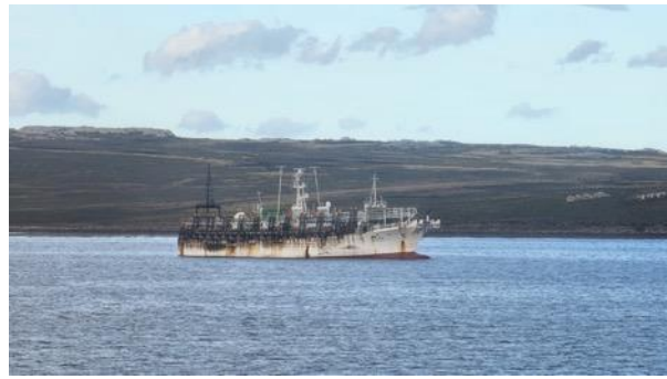
Photo 27-Korean squid jigger (which use light arrays to lure squid to the nets), Port Stanley, Falkland Islands
