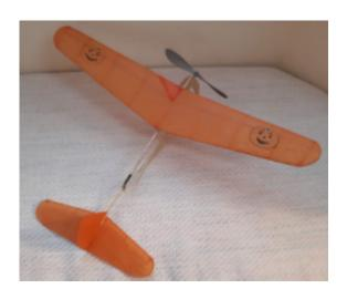
So that scratch-built Phantom Flash, like the other two models here, built easily. All were covered with gift-wrap tissue, way better than all but very expensive Japanese-made craft tissue Way Back Then. I used Avery's® permanent glue stick to apply it, and a light clear acrylic spray to seal and protect it.
