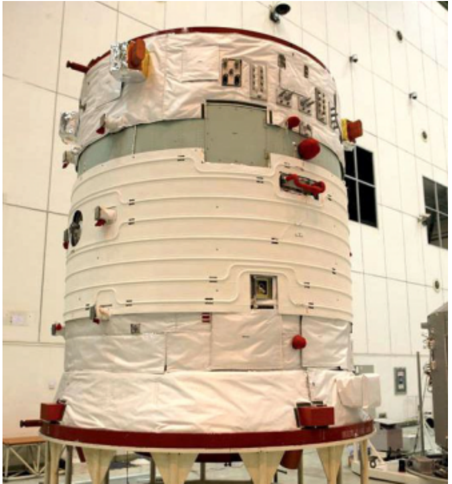
Shenzhou service module (via China Manned Space Engineering Office)
