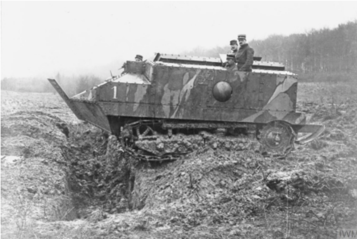
IWM Caption: "A French Schneider CA1 tank crossing a trench during training exercises. Note the camouflage the tank is covered with. Marly-le-Roi, December 1916. Source: IWM (Q 70321)"
