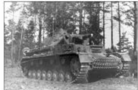
Above: In most respects, the Panzerkampfwagen Panther Ausf. C was similar to the Ausf. B, but the Ausf. C had an armored cover on the machine to protect the turret of the 7.5 cm KwC 2, a feature that is quite noticeable in this photo of a vehicle from the 1st Panzer Division. The "CB" symbol of that division is to the left of the turret's cover. On the right front of the turret, the armored cover of a machine gun is open. Patton Museum
