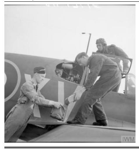
IWM caption: "Photographic staff transfer the film magazine of an Type F.24 aerial camera, mounted in the oblique position in a North American Mustang of No. 2
