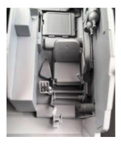
The interior of the hull is quite "busy" with a driver's seat and brake pedal, gear leavers etc. The driver's seat alone has
