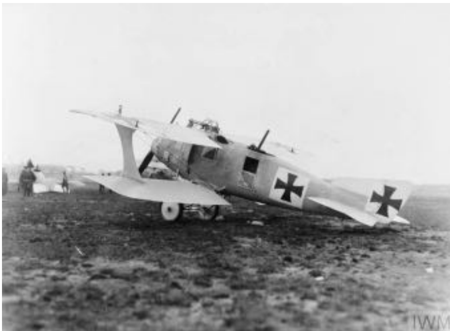
IWM caption: "LFG Roland C.II (Walfisch - Whale) two-seat reconnaissance biplane. Equipped with a fixed forward-firing machine gun." Source: IWM (Q 66683)
