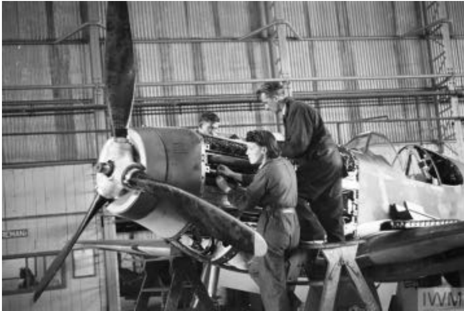
IWM caption: "Aircraft construction: The assembly of North American Mustang aircraft at the Lockheed Aircraft Corporation factory, Speke airport, Liverpool. The propeller is in position and mechanics (both men and women) are checking over the engine." Source: IWM (CH 6293)
