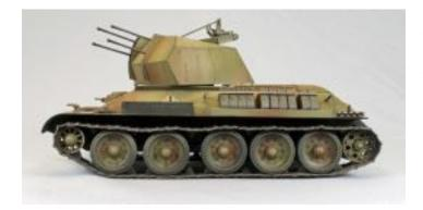
Future to seal them. Once dry, I carefully slipped the 20mm guns into the Flakvierling assembly and dropped that into the four base plates of the turret, a somewhat clumsy process. Once I had everything lined up however, it swiveled freely on the turret ring. I then airbrushed all the shiny areas with Vallejo Matt Varnish to prepare the vehicle for filters.
