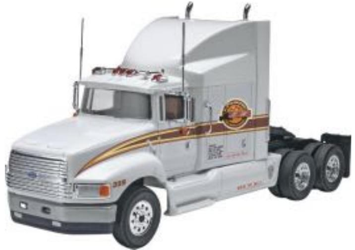
The cab roof and air dam are another single piece, and so is the rear cab wall. The front bumper (which includes a pair of fog lights) and side skirts are nicely done. Depending on how far you want to take a snap-together kit, you might opt to use your punch set to make the fuel tank caps, because the kit's detail is rudimentary.
