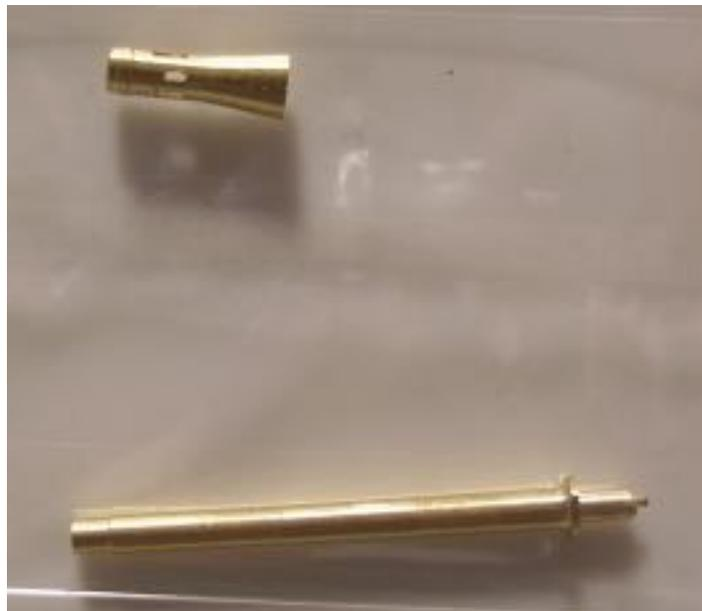
Assembly of the brass barrel is a snap. The cone slips tightly over the shaft and only requires a dot of super-glue to keep it in place.
