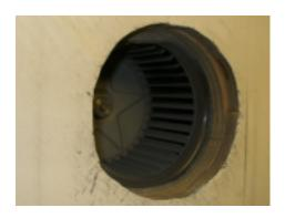
This is a close-up of the same hole shown above. The closer you match the hole to the intake of the blower, the stronger the current of air being drawn in will be. I put
