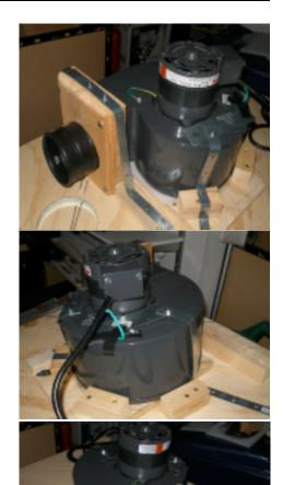
model! I used galvanized steel L fittings and some strong banding and bolts to secure everything. Once I was satisfied that the blower was not going to come loose short of being hit by a bomb, I set it aside and assembled the rest of the booth.
