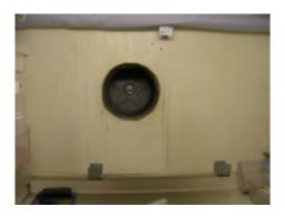
This is a picture from the front of the booth with the air filter removed, showing the hole cut in the back panel that matches the intake opening in the blower. The hole that I cut is slightly off-center to the left
