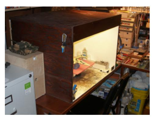
room. I cannot stress how well this design works (for me), while allowing for a smooth, horizontal air flow from my airbrush directly out the back of the booth. I used a 345hp Grainger blower, venting the exhaust via a laundry-dryer hose through the wall behind the booth. The outside opening in my garage is covered with a flapper valve. Everything is out of sight and out of mind.
