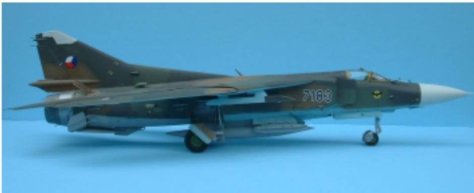
The last addition to the cockpit area was a significant amount of epoxy putty packed into the nose. There is a lot of plastic aft of the kit's center of gravity, especially with the wings in the swept back condition so I didn't want a tail sitter. I filled most of the nose forward of the cockpit with putty.
