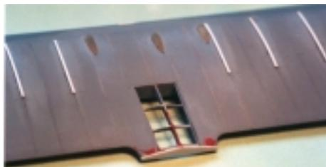
Scribed reinforcing patches around the holes drilled for aileron control cables and around the wing tank drains and cabin air intake.
