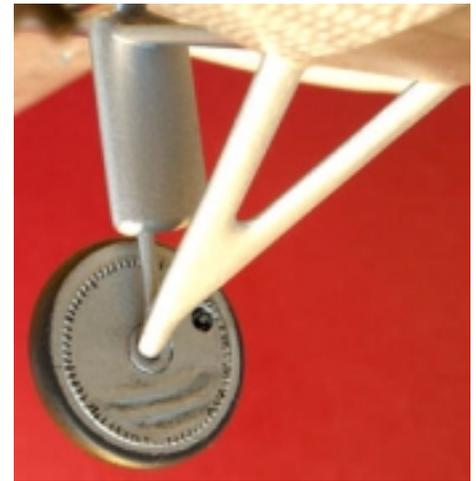
Replaced the tubular lower members of the LG with brass rods for strength.
