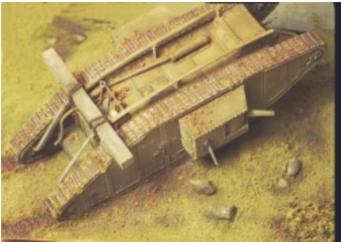
De-ditching beam, exhaust pipe and clumps of mud/grass on tracks.
