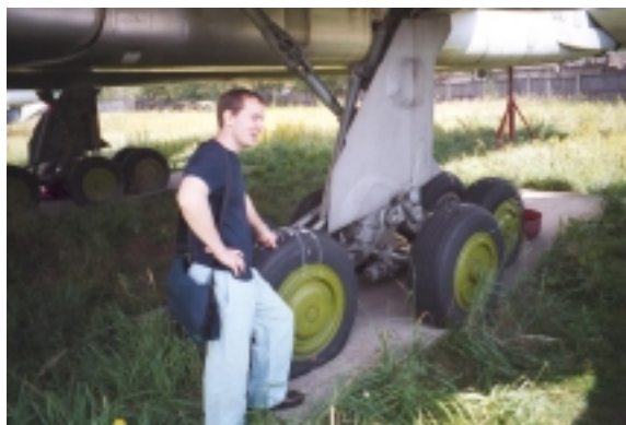
Fig. 8 – Tu-22M “Backfire” main landing gear, with formerly secret wide footprint bogies for operation on unimproved runways. As this photo was taken, my friend Sergei (a 737 pilot at Transaero) was saying, “Now that I have shown you this, I will have to kill you.”
