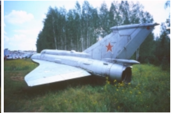
Fig. 6 – MiG-21I, a delta wing test bed used during Tu-144 development.
