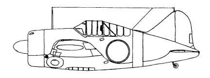
Note: Relocate exhaust to body from cowl
