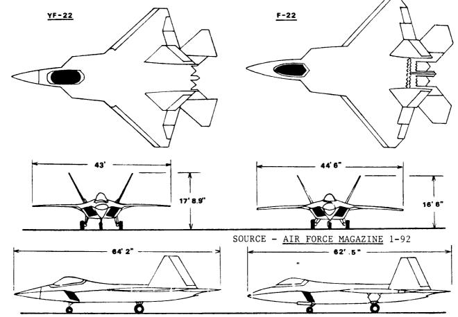
Cockpit more forward, lower canopy, intakes aft a bit, NLG & MLG both aft a bit & shorter, less wing sweep & more wing area, smaller tailfeathers, anhedral in the wing and exhaust nozzles more rounded.
