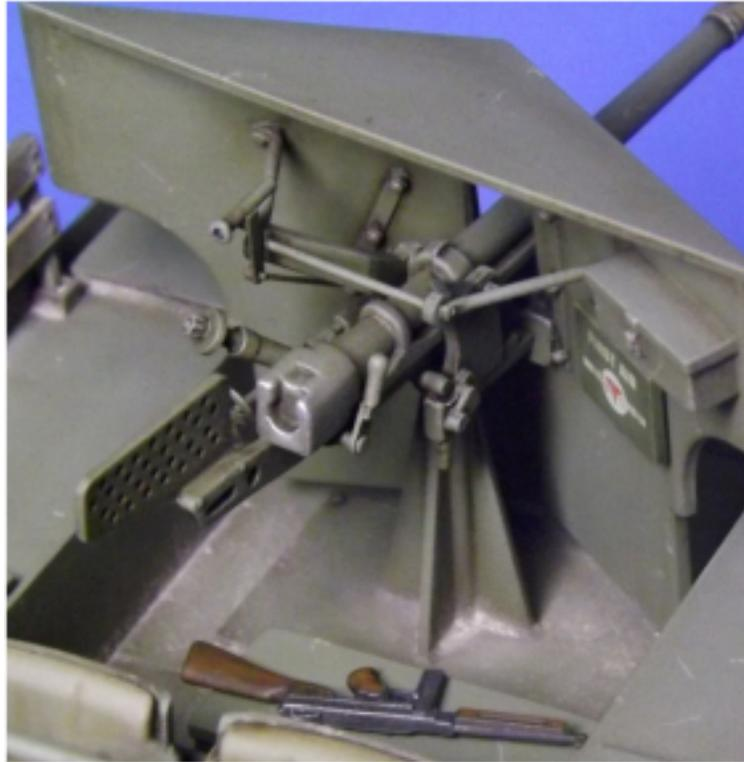
The front of the shield was sanded smooth to accept the bolts and attaching rivets for the tool box. These were made with the punch set from Historex. I kept the rivet and bolt lines straight by using tape as a 'flexible ruler'. I used the kit tool box.
