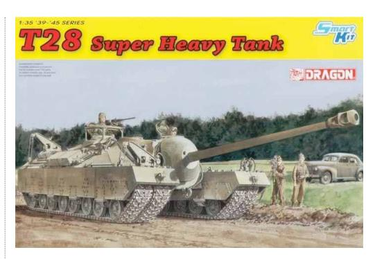
The frontal armor was up to 305mm thick, sufficient to withstand the famed German 8.8cm cannon. To cope with the immense weight, the vehicle ran on four sets of tracks instead of the usual two. However, its 500hp engine was underpowered to handle such bulk, meaning the T28 was slow (a 13km/h top speed) and cumbersome (military bridges of the day could not bear its weight). It was to operate with a four-man crew.
