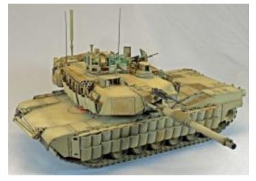
hitting on the vulnerable sides, rear, top, and underneath the tank. These problems have been partially resolved by fitting the Abrams with the Tank Urban Survivability Kit (TUSK). This field-installed kit was developed to improve survivability and situational awareness when operating in the close confines of a city. Introduced in 2006, the TUSKs (in one form or another) found their way to all tanks fielded in Iraq by 2008.
