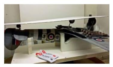
I had no choice but to move on. I drilled out the holes in the wheels, slipped the wheels on and filled the spaces with 2-part epoxy. While the epoxy was drying, I balanced a piece of flat cardboard on all three wheels to assist in lining up the 'flat' spots so they would sit properly on a table top when the model was set on its wheels.
