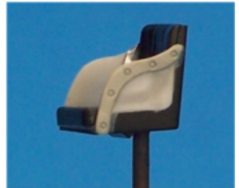
Close-up of the seat. Note the detail pressed into the seat cushion arm. This was done with a piece of rod with a hole drilled in it. I dipped it in water so it wouldn't stick to the soft putty.
