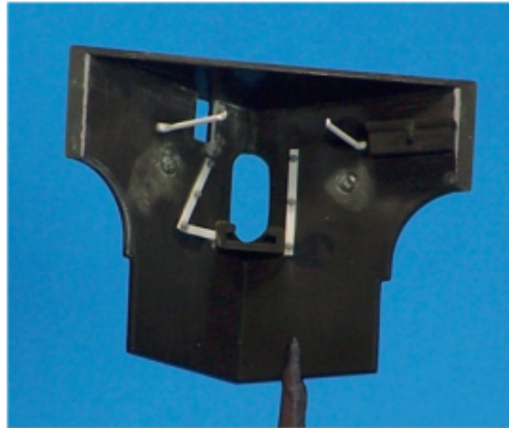
View of the rear of the gun shield. Note the large ejector-pin marks and large pits for the kit shield supports.
