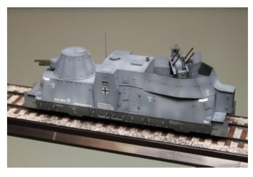
separate compartment for the single-piece upper section of the rolling stock. The parts are crisp and flash-free, and effort has been made to restrict the many ejector pin marks to areas that are not visible from the outside. The flak gun platform and the protective armor around the car-coupling hardware are the only areas that will need these marks cleaned up. The plastic is soft and sands easily.
