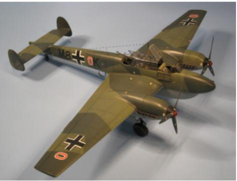
against each wing half. I had to add some thin strips of plastic card to one wing half to correctly align its corresponding nacelle. The other nacelle was better aligned but still left a significant gap on the upper surface join. Although the adjustments and need for filler were hardly unusual, it came as a bit of a surprise with the Eduard kit. Previous Eduard builds had resulted in next to no filler in any of the major joins.
