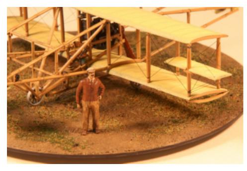
cutting to shape, then affixing to the underlying styrene structure by judicious application of liquid solvent cement. The softened styrene works its way up into the aeroskin fibers, and forms a surprisingly strong bond when it hardens. Working from the middle out on each surface, you keep it as taut as possible and trim off the excess with a sharp blade when dry.
