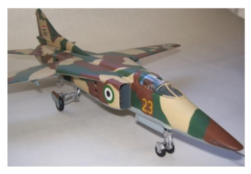
The machine is fitted with a ventral fin, low near the back of the fuselage, and more than half of its area folds sideways for landing. On this kit, the two parts are a press fit together, with no hinging or other mechanism.
