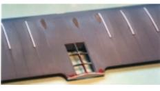
Scribed reinforcing patches around the holes drilled for aileron control cables and around the wing tank drains and cabin air intake.
