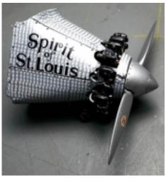
Replaced plastic push rod tubes with metal rods.
