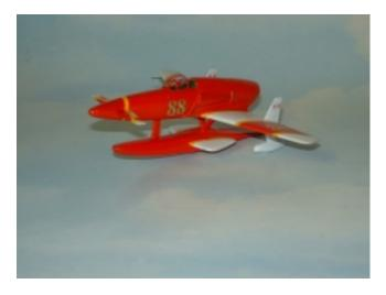
Model Information: The kit is Hasegawa's "jet" offering of their basic Shindenkai kit. It comes with a replacement tail cone and slightly larger intakes. The float was my first attempt to make resin copies of the Matchbox Twin Otter float. I ended up with most of a float with a big air bubble in the back. Rather than toss the incomplete float, I thought it would look
